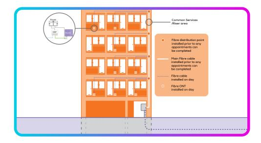
Each apartment/flat is designated an internal fibre from their ONT to the floor riser where other services are normally supplied from.
